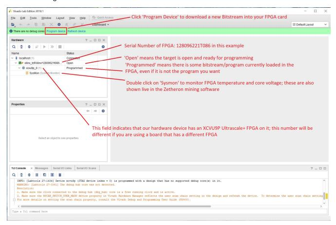
At this point it is a very good idea to take a piece of masking tape, stick it onto the FPGA card and write down the serial number on the masking tape. Make sure only one FPGA card USB cable is plugged into your computer, so that you know that the serial number being displayed is the one corresponding to the single card plugged into your computer. You can plug one card into your computer at a time, and you will see the serial number in Vivado Lab Edition, so you can enumerate all your cards:
