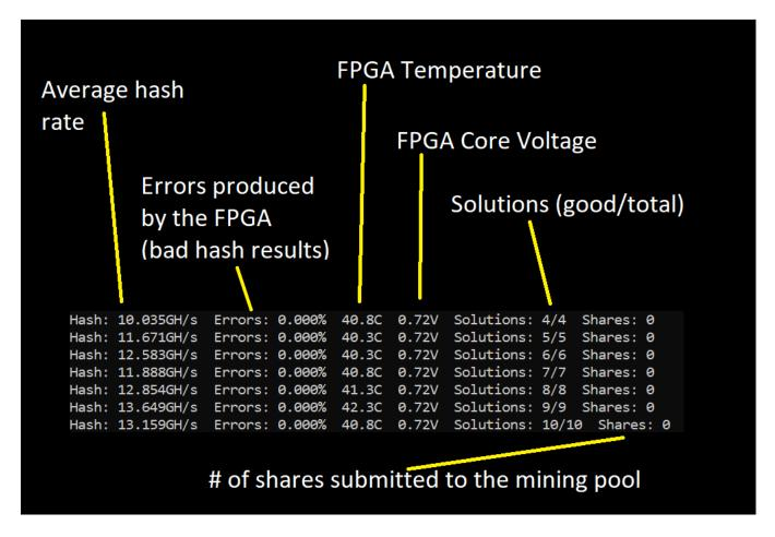
The average hash rate is the rate of 'valid' hashes, after errors have been subtracted. The FPGA temperature is important; if the temperature goes over 92C, there is a risk of the card shutting down. If the VCU1525 overheats, the mining software will no longer produce any solutions, and if you have a Vivado Lab Edition window open, you might see the following image:
